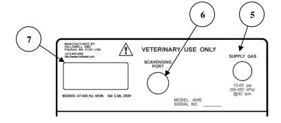
connector. The scavenging port will accept either the 19mm scavenger tubing or a 15mm ET adapter. The electrical power inlet is the standard IEC320 connector. The power supply in the AWS is a universal supply that will accept any standard power source as noted on the rear panel.
