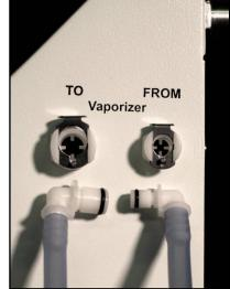
of 1/4" ID tubing, not supplied, and connect the larger quick connect to an FS-2A vaporizer inlet connector and the smaller quick connect to an FS-2 vaporizer outlet connector.
