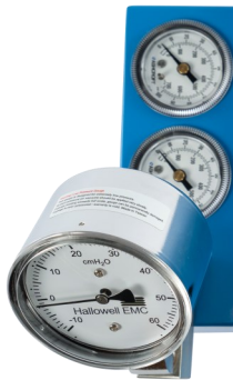
Panel Gauges show Air and O 2 psi from supply hoses.
