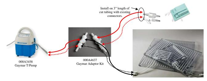
The Hallowell EMC Hard Pad has been designed to be used with existing heat therapy systems such as the Gaymar T/Pump®, HTP-1500 and Hamilton Pump. *Follow the instructions in your specific operator's manual in regards to startup, shutdown, storage, draining and cleaning instructions.*
